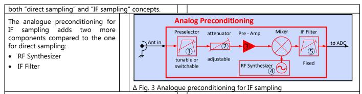
IF sampling concepts may be the better choice compared to direct sampling in cases where strong interferers are very close to the wanted frequency. In this case the pre-selector filter may not be able to provide a sufficient selectivity to suppress the interferer in a way that the complete spectrum at the input of the ADC is within the operating window of the ADC.
