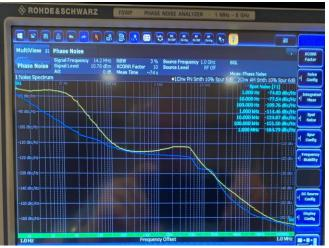
$\Delta$  Fig. 13 Phase noise of an analogue Transmitter
