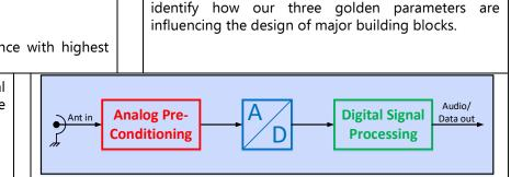
$\Delta$  Fig. 1 General and simplified SDR architecture
