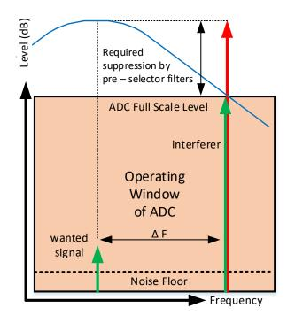
$\Delta$  Fig. 8 ADC Operating Window with Pre - Selector These easy facts are now giving a clear advice which concept to be used or is best for an SDR HF receiver.
