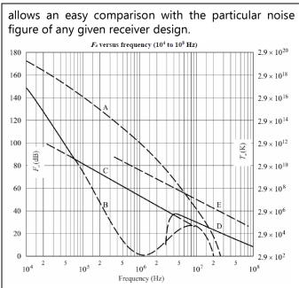
$\Delta$  Fig. 6 Noise external to an HF receiver
