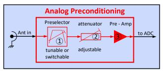
$\Delta$  Fig. 2 Analogue preconditioning for direct sampling
